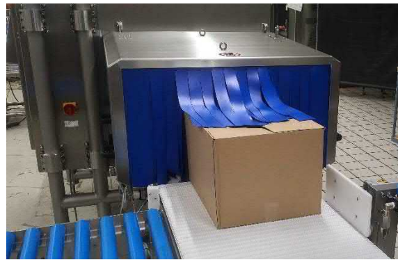
Double layer of protective curtains for safe working near the XRAY SHARK®.
