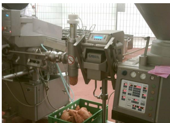
METAL SHARK® IN Meat fitted into a production line.
