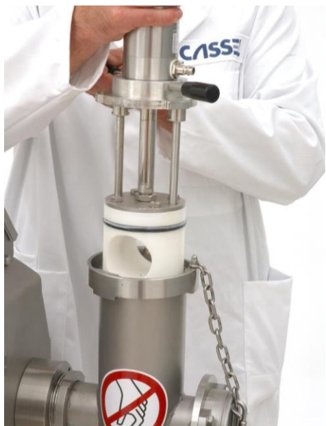
Piston valve for reliable discharge of contaminated product parts.
